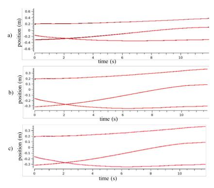
Fig. 16 Desired (black) and obtained 3D trajectory (red) during the tracking. a) Equation (37). b) Equation
