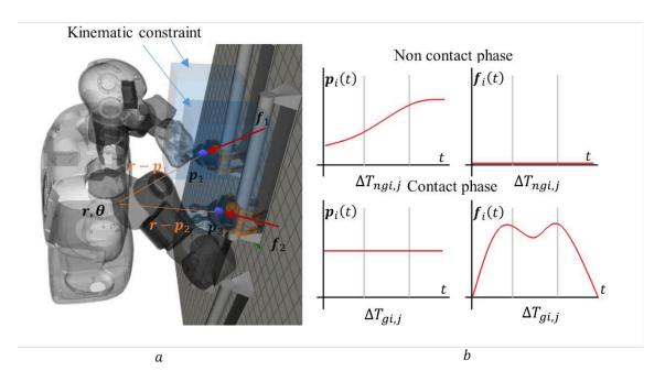
Fig. 2 a) 3D representation of the robot, contact forces and kinematic constraint. b) Example of end-effector position and force during non-contact and contact phases.
