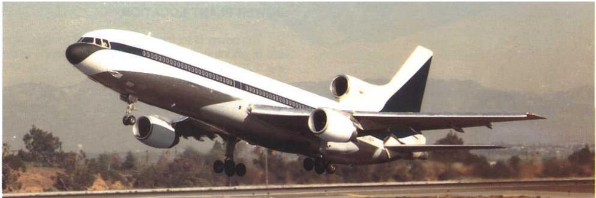
Figure 2-2 Tail and Wing-Mounted Pod Installation [7]
