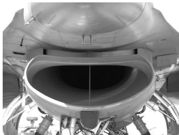
Figure 3-4 Fixed Geometry Intake on the F-16 Aircraft [53]
