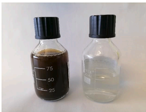
Fig. B2. Photo of wastewater centrate from an advanced anaerobic digester (left) and recovered ammonia distillate (right).
