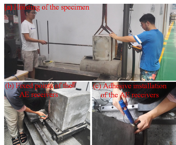
Fig. 2. Hoisting of test specimens as well as fixed points and the adhesive installation of the AE receivers.
