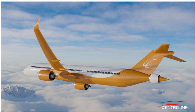
Fig. 1. Artist's Impression of the CENTRELINE turbo-electric propulsive fuselage aircraft design.
