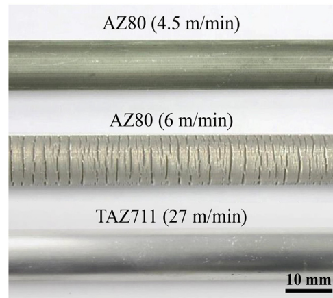
Fig. 7. Photo shows quality of surface in AZ80 and TAZ711 extrusions (350 °C) [169].
