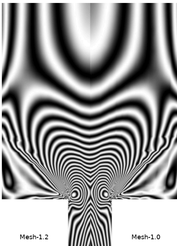
Fig. 16. Simulated birefringence patterns using the main mesh (Mesh-1.0) and the finer mesh (Mesh-1.2). Both are produced with a stress optical coefficient of 1.18 \times 10^{-9} \text{m}^2/\text{N} .
