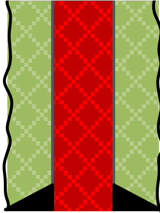
Figure 2.10: Example of External and Internal WBEs at Casing Shoe (External WBE in Green; Internal WBE in Red)
