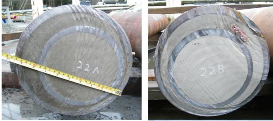
Figure 4.3: Expandable Cement Cut, No Control Lines (left) and Control Lines (right) (Aas B. et al. 2016, figure 11)
