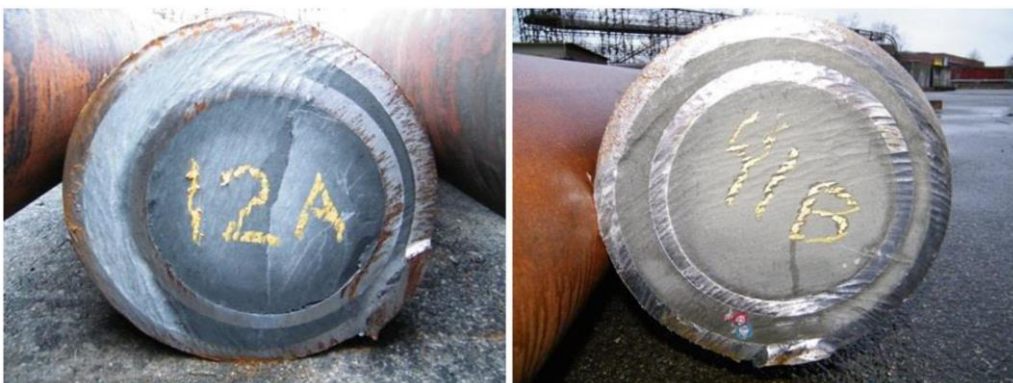
Figure 4.2: Portland Cement Cut, No Control Lines (left) and Control Lines (right) (Aas B. et al. 2016, figure 9)
