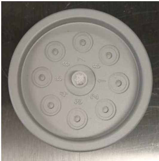
Image 2. Residual sample after TGA-measurement.
