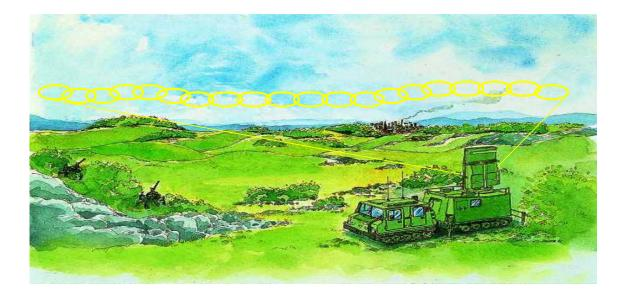
Figure 2.3: The search pattern of a WLR (in yellow) shows that a sector of the horizon is searched. This typically happens several times every second to detect projectiles emerging over the horizon. To avoid ground clutter, the search is performed slightly above the actual horizon. Image source: Saab.
