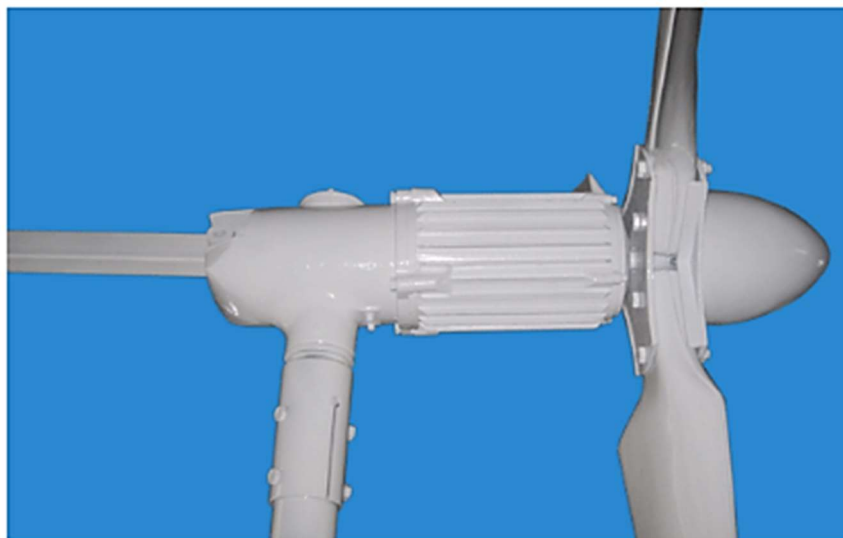
5.4 Assemble the tail rod and fix to the rotor body by a stainless steel pin roll. The Pin roll could be pull out by a M8 bolt.
