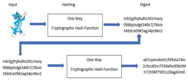
Figure 2. Concept of One-Way function operates
