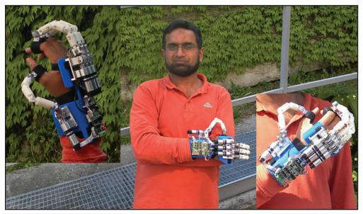
A lightweight, flexible, under-actuated exoskeleton hand has been created in work from the Italian Institute of Technology (IIT), Genova, Italy. Intended as a general purpose device, the four-finger design is now being explored as a medical rehabilitation aid but has wide potential from assisted living to virtual reality.
