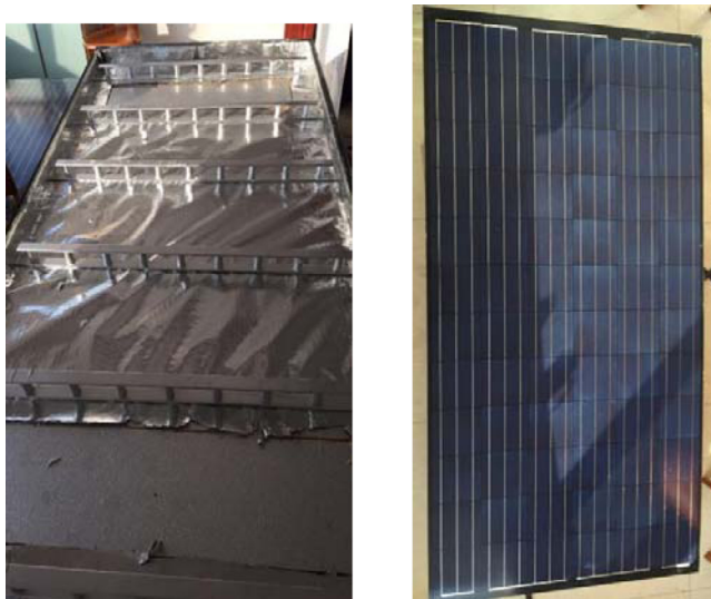
Fig. 3. Picture of the mini-channel PV/T panel.
