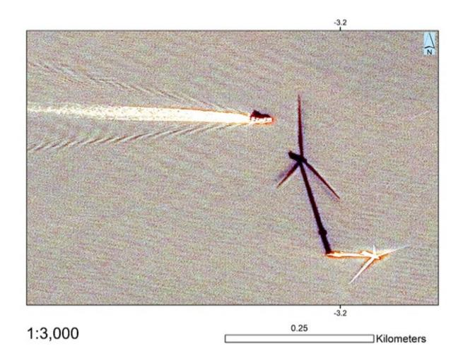
Figure 8: High-resolution Pleiades image with  $0.5~\mathrm{m}$  pixel size showing details of an individual wind turbine and passing crew transfer vessel.
