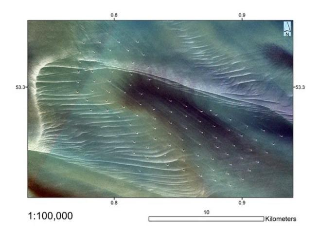
Figure 7: Medium–resolution Sentinel–2 view of 580 MW Race Bank offshore wind farm showing details of underlying seabed bathymetry during a period of calm weather and transparent water. 91 wind turbines are visible within the farm, with some in shallow water (< 15 m, lighter colour) located on rolling sand wave structures, and others in deep water (> 20 m, darker colour) where seabed details are not visible.
