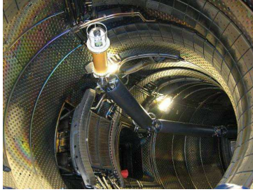
Fig. 9. AIA with the viewing system inside Tore Supra tokamak
