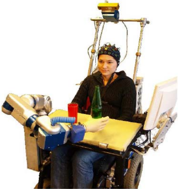
Figure 2. SSVEP based BCI control of a three dimensional robot. [9]
