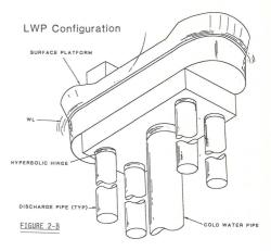
For both the SWP and the LWP, a fiberglass-reinforced plastic/syntactic foam sandwich with stiffening rings placed along its length was chosen as the best CWP design. Both configurations also used a multileg catenary mooring system, because it provides the lowest technical risk and also accommodates depth changes of the transitional platform between surface, operational, and deep depths.
