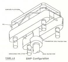
At the start of the study, the capability to decouple platform motions from the CWP through the use of a flexible or gimballed transition CWP was viewed as a possible means of reducing the loads on (and thus the risk to) the CWP. But as the
