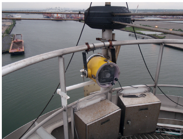
FIG. 2. A Nikon D-200 10-MP camera with an AF Nikkor 180-mm f/2.8D IF-ED lens placed in an Ocean Images underwater housing unit installed on the aft mast of the Explorer of the Seas (Fig. 1, location B).
