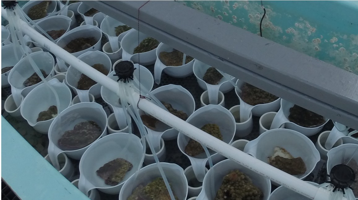
Figure 1: Recirculating aquaria system with adult colonies of Porites astreoides . Rubber tubing regulates water flow and water pressure to assure ideal oxygen distribution. The water leads to PVC pipes fitted with plankton mesh to sieve out planulae.
