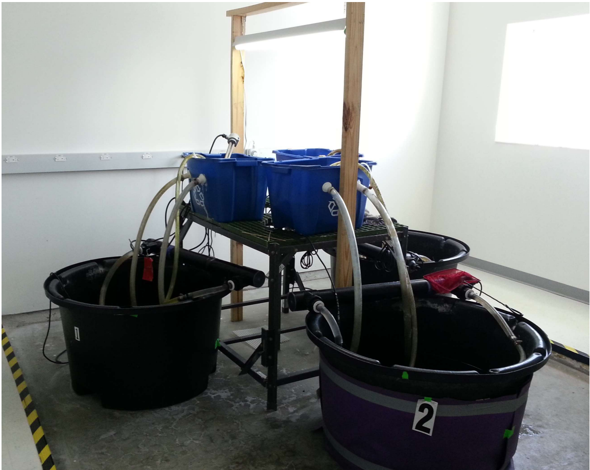
Figure 1. Photo of the quarantine tanks. Black tubes on tanks are UV filtration units. Blue bins are sumps containing biofiltration media and overflow back into the main tanks. All three tank systems are isolated from each other
