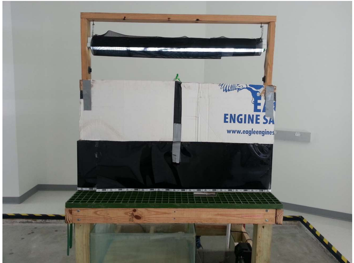
Figure 2. Photo of the experimental tanks in testing mode. Image includes the restricted light bar, GoPro mounting brackets, and cardboard divider.
