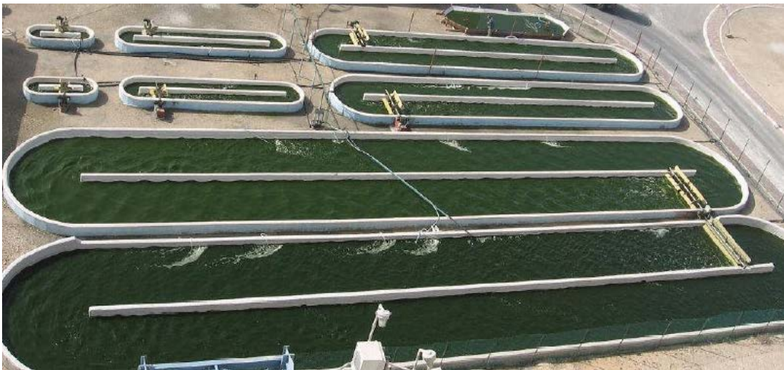
Figure 7. Example of oval production tanks at Israel Electric Company in Ashkelon, Israel (from National Renewable Energy Laboratory; www.NREL.gov )
