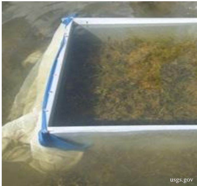
Figure 5. Throw-trap used for sampling fish and invertebrates associated with the seagrass canopy. Curtain nets located on two parallel sides of the trap covered between sweeps to prevent animals from escaping.
