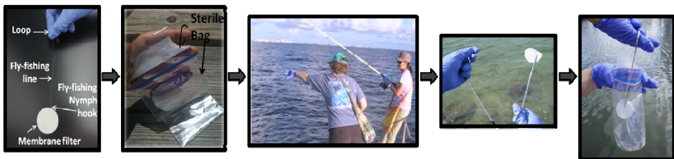
Figure 3.2: Sampling technique developed for the sea surface microlayer.
