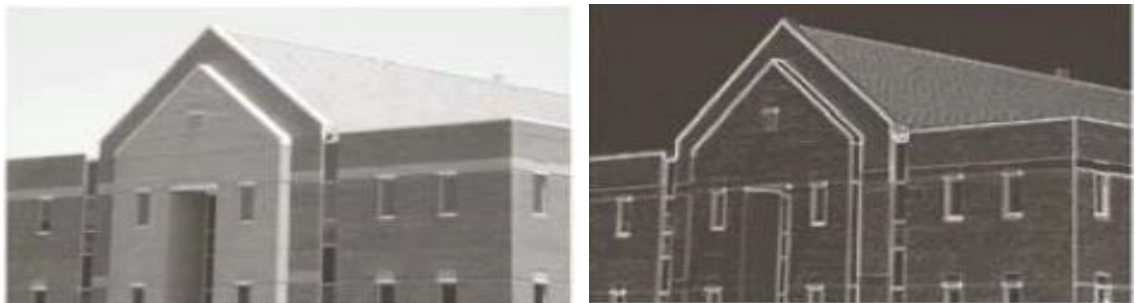
(a) (b) Figure 7. Edge detection example (Kunt et al., 1985), (a) Original picture of an M.I.T. Building, and (b) After applying the Sobel operators.
