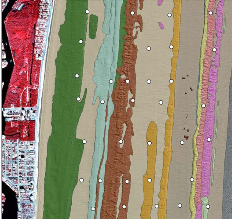
Figure 49: Example of the accuracy assessment point grid off Hugh-Taylor-Birch State Park in central Broward County.
