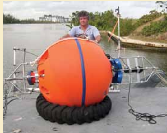
Associate Professor Alexander Soloviev, Ph.D., with state-of-the-art acoustic Doppler current profiler (ADCP) mooring developed and maintained by the Physical Oceanography Lab in the Florida Straits since January 2007
