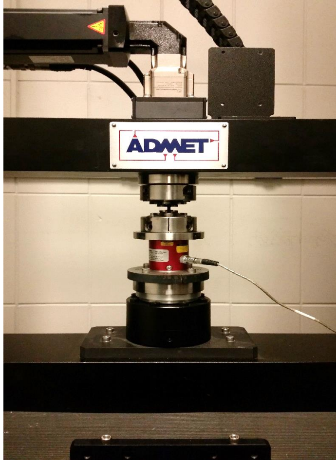
Figure 32: A photograph of the ADMET testing system showing two load cells stacked on each other.
