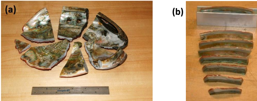
Figure 27: Cutting up the shell into segments (a), and then strips (b).
