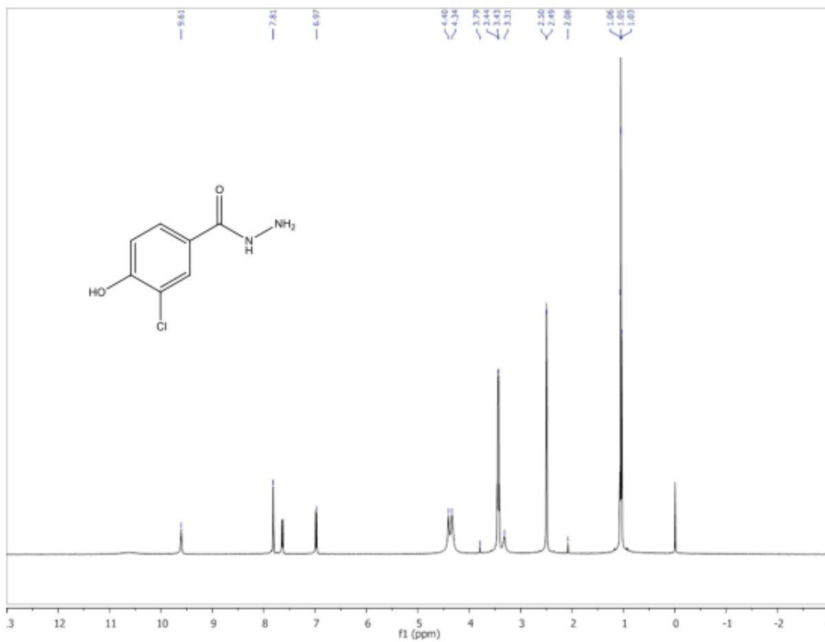
1 H NMR Analysis of 3-Chloro-4-Hydrobenzohydrazide (3)
