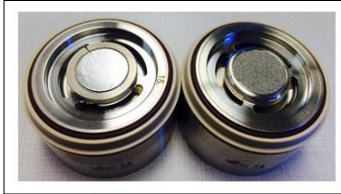
Figure 5.2 (Left) ELPI smooth plates (right) ELPI sintered plates
