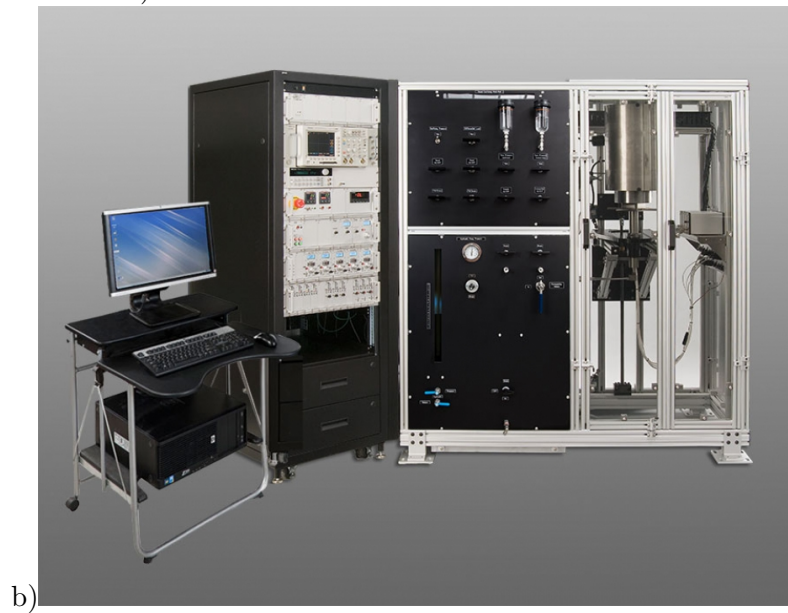
Figure 3.7: a) Prepared core/core holder assembly mounted to base plug of vessel b) Autolab 1500
