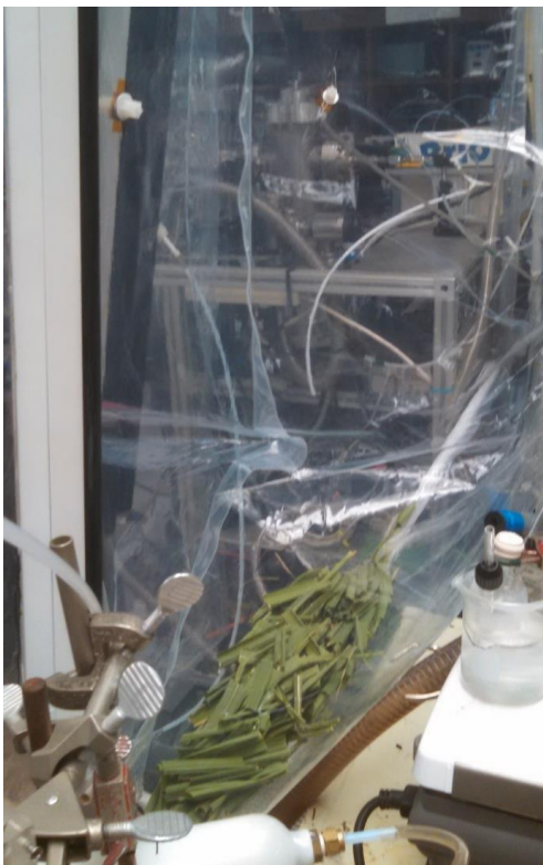
Figure 8.1 Sugarcane in 775-L reaction chamber for emission and SOA yield experiments.
