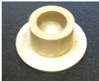
Figure 4.2: Additively manufactured aluminum "chalice" used during the experimental drop tests. The diameter and depth of the "chalice" are both 15.875 mm.
