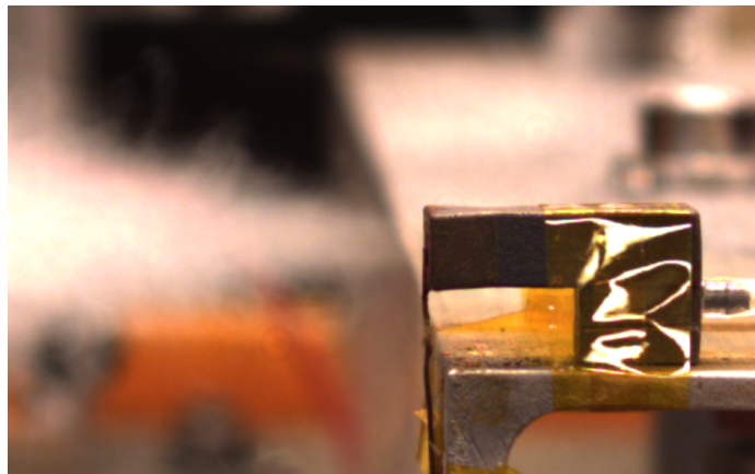
Figure 5.15: A photograph of the thruster system operating during the plume temperature measurement experiment. Condensation surrounding the plume is visible.
