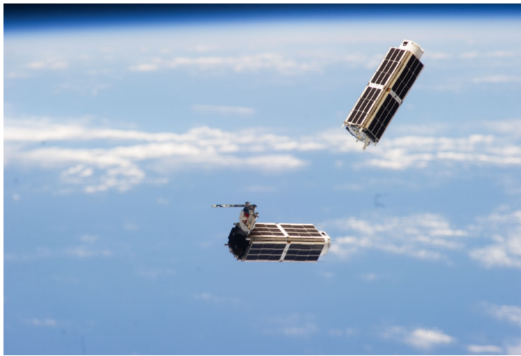
Figure 1.2: Two of 28 CubeSats deployed as part of a CubeSat constellation called Flock 1 from the International Space Station in February 2014. These CubeSats did not have propulsion systems and were expected to re-enter after three to five months. Reproduced from [11].
