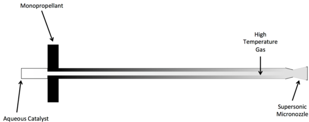
Figure 1.5: Schematic of the homogeneous catalysis concept. The monopropellant is brought into contact with an aqueous catalyst in a specially designed mixing chamber, which results in rapid, exothermic decomposition. The resulting products are vaporized and ejected through a converging-diverging nozzle to generate thrust. Reproduced from [38].
