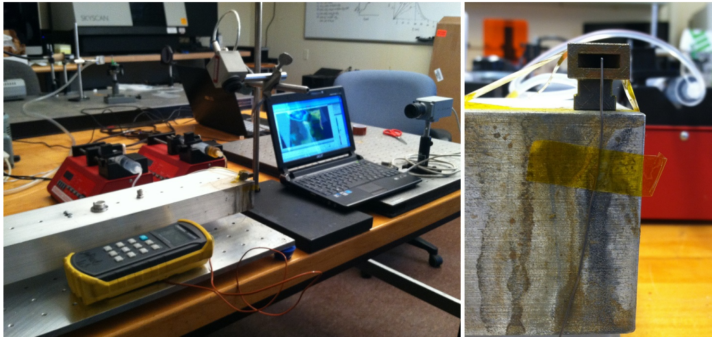
Figure 5.14: Right: Photograph of DMLS titanium nozzle used for plume temperature measurement. A type K thermocouple was placed directly in the center of the nozzle exit for temperature measurements. Left: Photograph of entire experimental set-up including thermal imaging camera, video camera, and digital thermometer.
