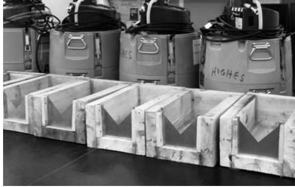
Figure 5. 90-degree thin plate v-notch weirs (foreground)
