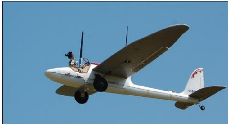
Figure 1 Multiplex “Easy Star” with wireless camera system
