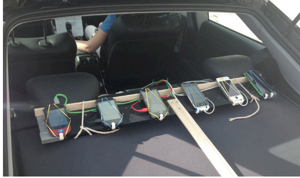
Figure 24: Smartphones securely mounted in the trunk of a hatchback vehicle.
