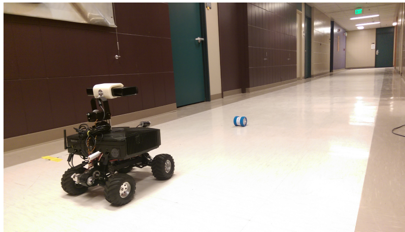
Figure 5.2: Robot setup for multipath (hallway) RSSI sampling experiment.
