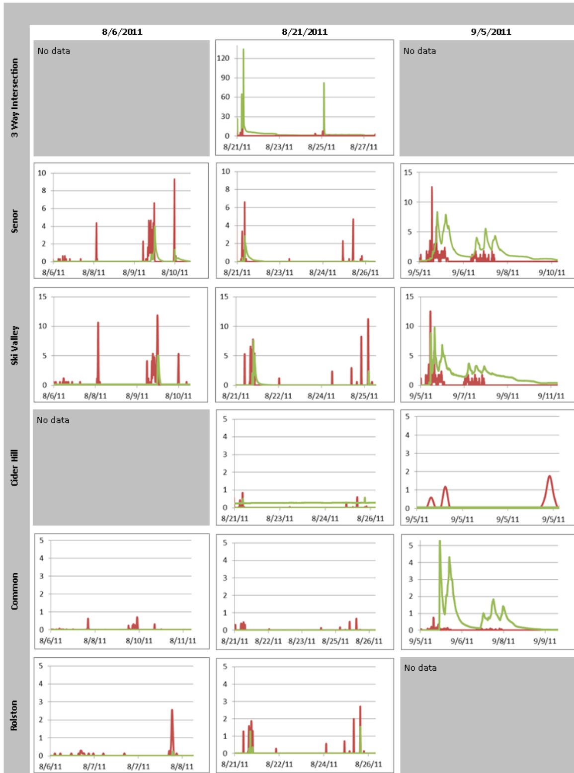
Figure 4: Graphs illustrating total measured runoff (L/sec) in green lines and simulated road surface runoff (L/sec) in red lines using the rational method for selected storms and sites monitored during Summer 2011.
