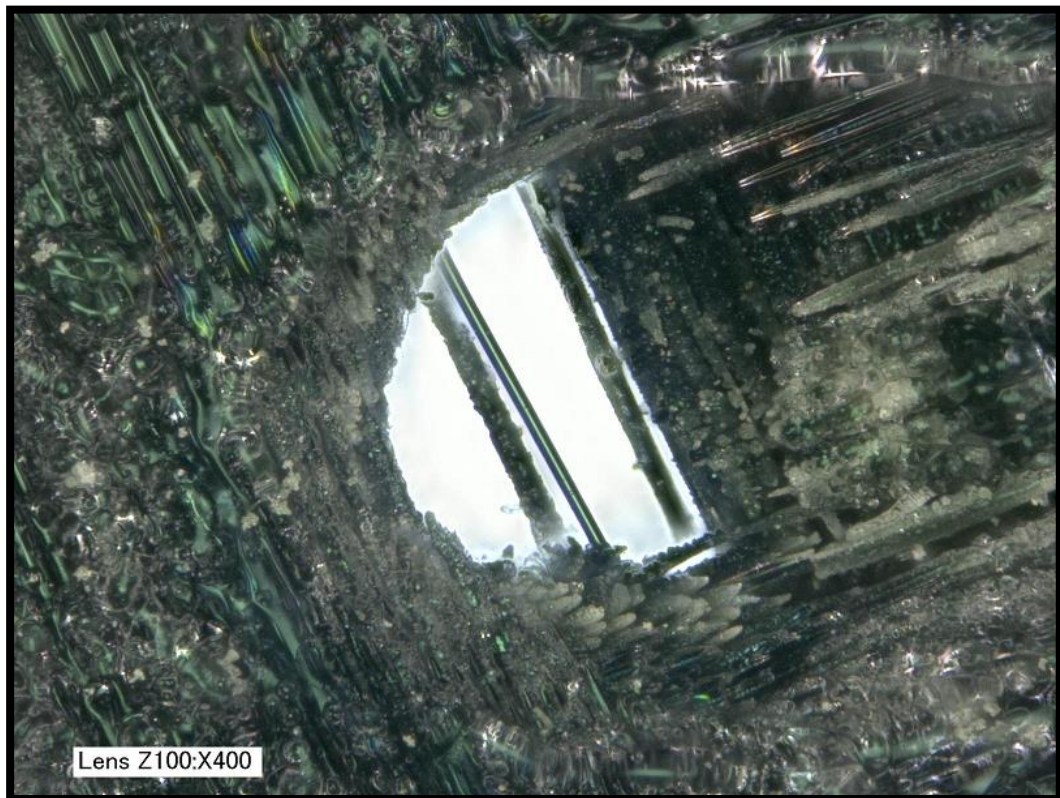
Figure 60: Keyence image of a location of catastrophic failure showing worm holes typical of failure in oxidizing plasmas
