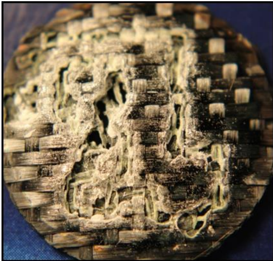
Figure 56: Coupon image of failed sample after less than 10 minutes of air plasma exposure
