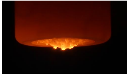
Appendix F.1: Profile image of the pre-gashed SiC fabric sample taken during exposure to an air plasma
