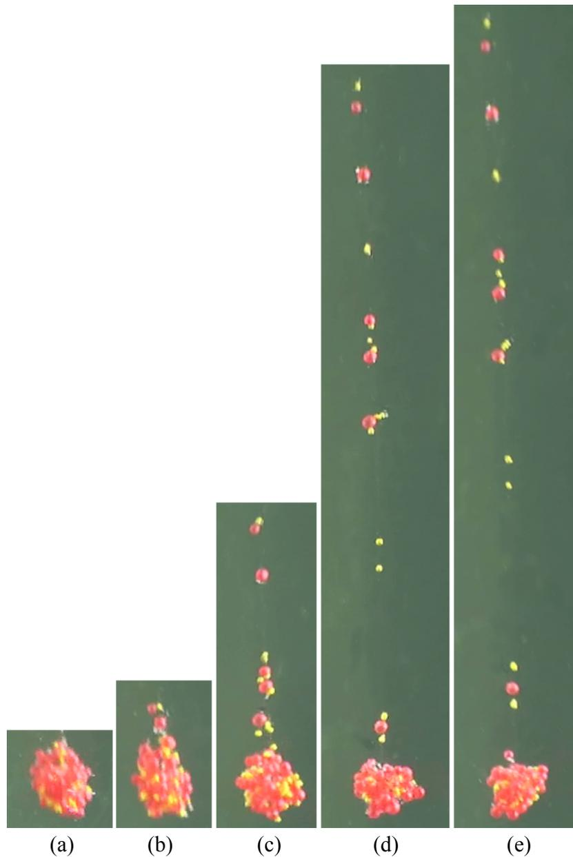
Figure 36: Photo of the particle positions of a falling droplet, with initial droplet diameter  $d_d = 3.8$  mm, in experimental set 1 at times (seconds): (a)  $t = 0$  , (b)  $t = 0.8$  , (c)  $t = 1.8$  , (d)  $t = 3.8$  , and (e)  $t = 4.3$  . The large particles (red) are about 2.2 times larger than the small particles (gold).
