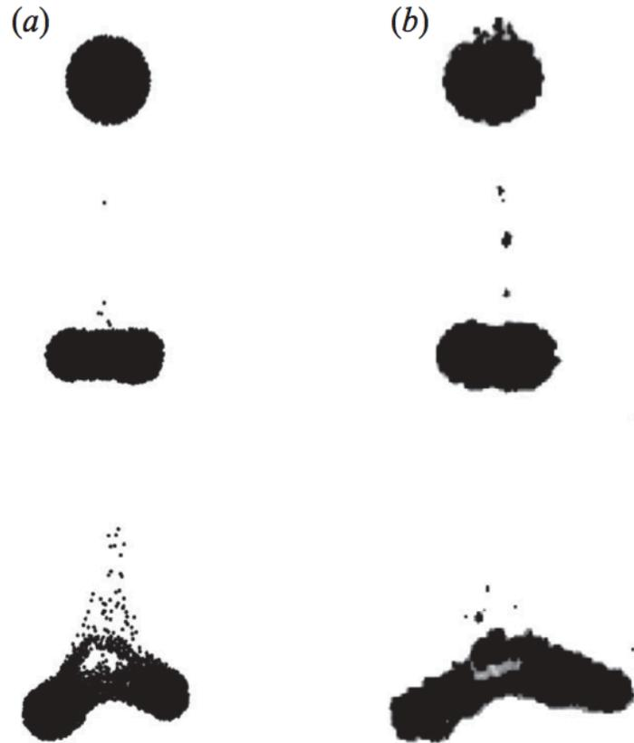
Figure 7: Typical evolution of a falling suspension droplet in the micro-scale inertia regime where  $l^* \approx 20$  and there is significant particle leakage. (a) Oseenlet simulations with  $N = 7500$  and  $l^* = 20$ , (b) experimental results with  $N = 7000$ ,  $Re_d = 3.5$ , and  $l^* = 21$  (From Pignatel et al., 2011).
