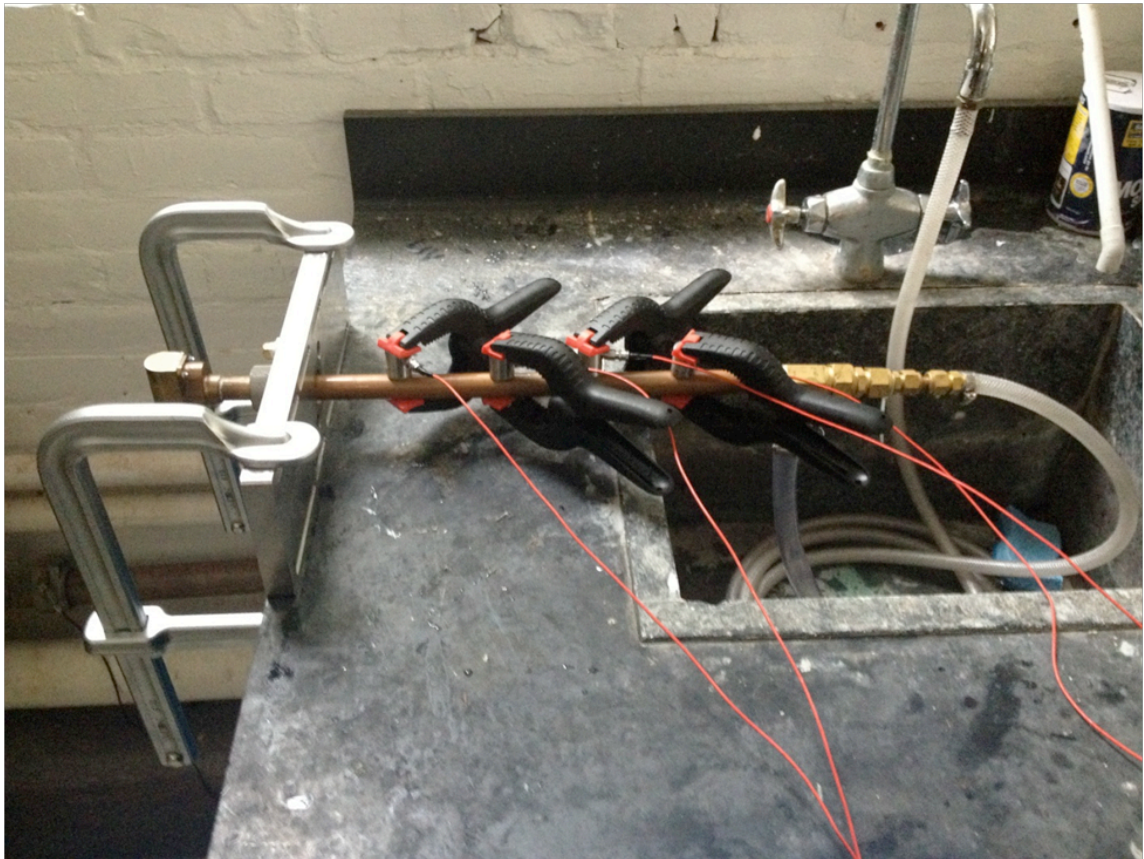
Figure 10: Four sensors spaced evenly along the copper pipe of water-cooled waveguide
