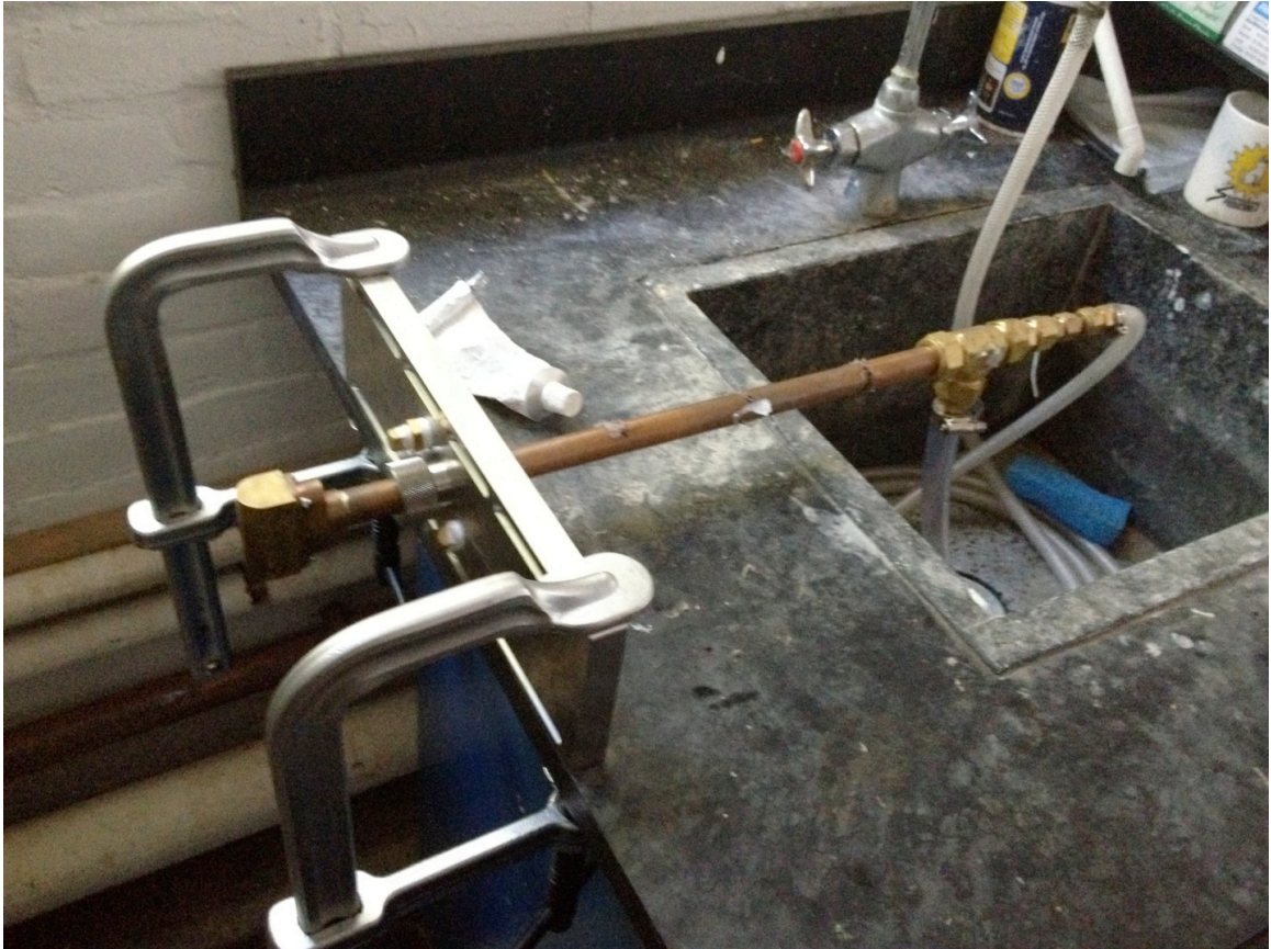
Figure 8: The water-cooled waveguide firmly clamped to a granite counter with its water intake connected to a faucet and an “exhaust” tube down the drain
