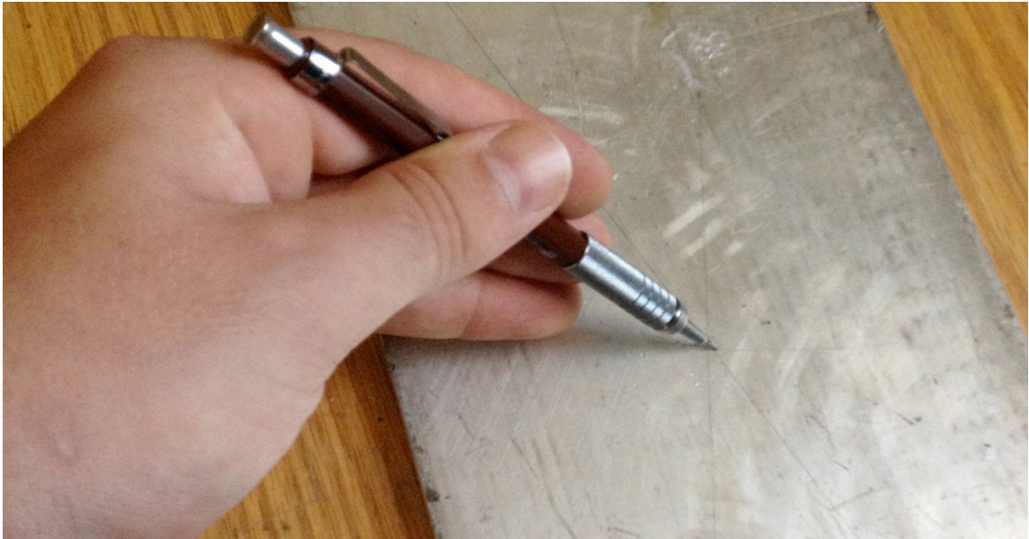
Figure 3: Demonstration of a pencil lead test; note, hand is elevated from plate
