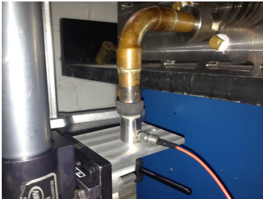
Figure 18: Actuated sensors placed firmly against the graphite sample
