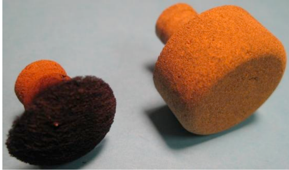
Figure 1: Test samples for monitoring material performance in a high temperature plasma stream [2]
