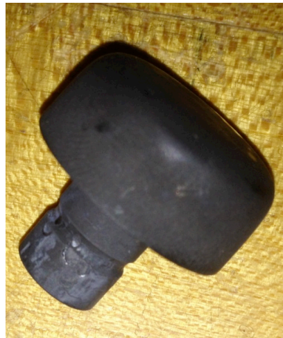
Figure 16: The graphite sample from figure 15 out of the holder
