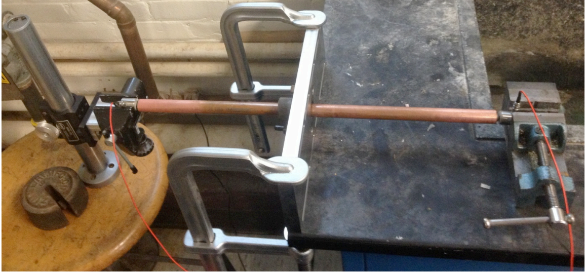
Figure 45: The experimental setup with actuating transducer, left; and sensing transducer, right
