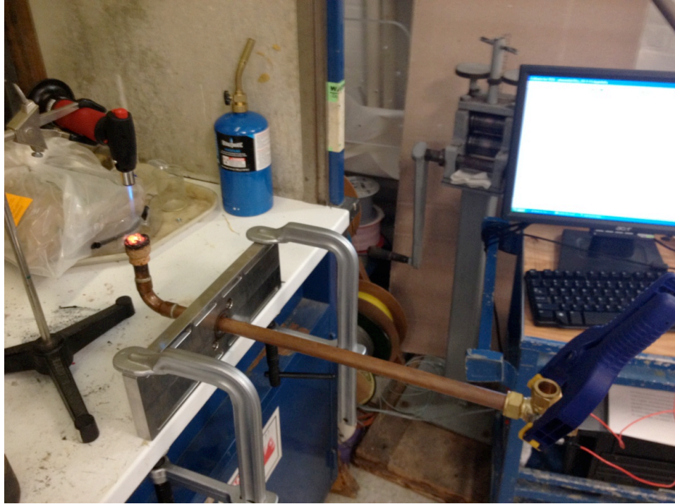
Figure 23: The butane torch is applied to cork sample while AEWIn is collecting data
