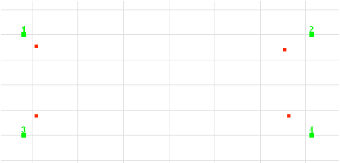
Figure 7: Four lead breaks in rectangular formation near the sensors
