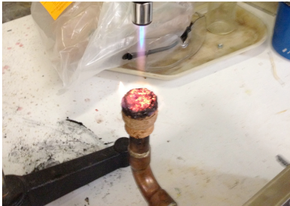
Figure 24: Close up of the burning cork sample
