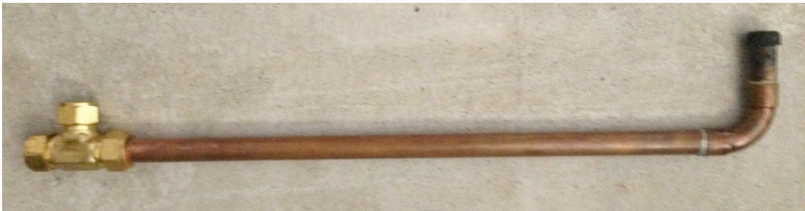
Figure 15: Waveguide 2 with a graphite sample in the holder, right
