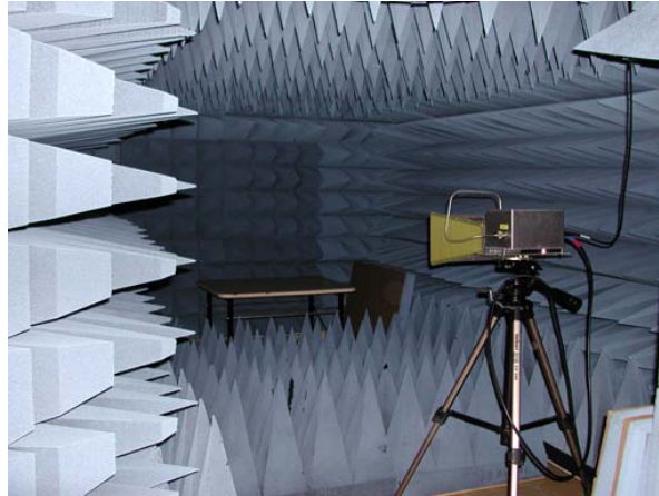
Figure 7.1. Anechoic chamber testing a horn antenna 2
