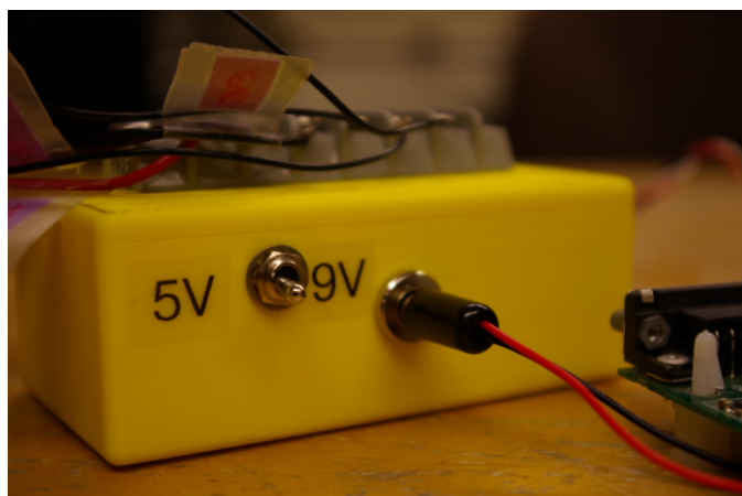
Figure C.2. Latest version of antenna power supply
