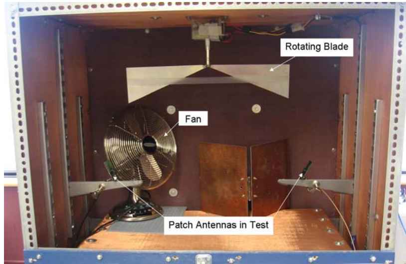
Figure 7.3. Fabricated CRCE with oscillating fan
