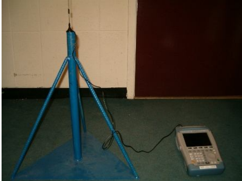
Figure 23. Receiving antenna and spectrum analyzer
