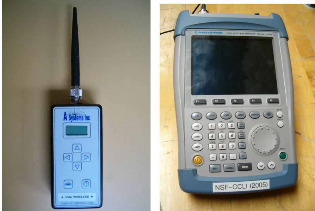
(a) Transmitter: A System Inc signal generator (b) Receiving spectrum analyzer: Rohde & Schwarz FSH6 spectrum analyzer
