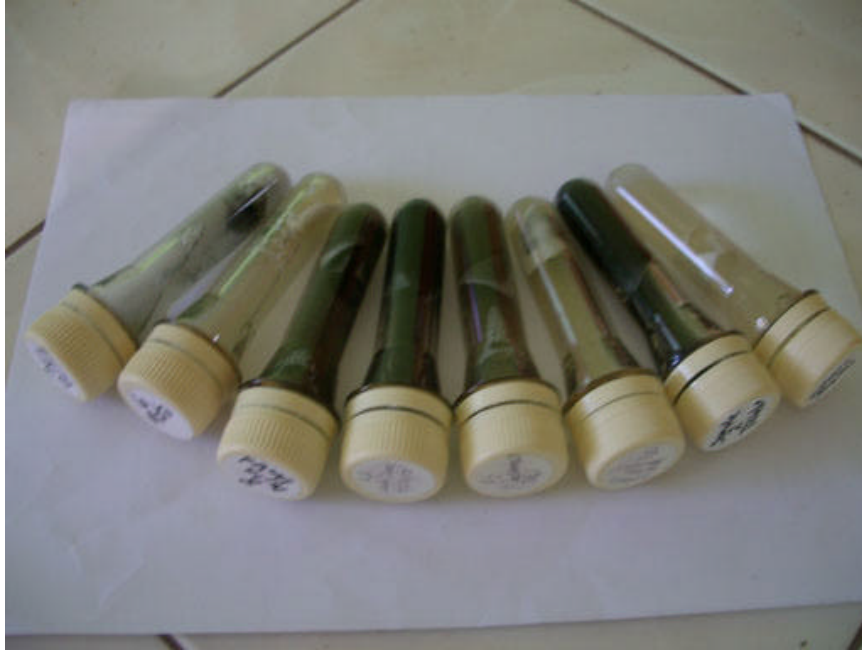
Figure 3: Paper Strip Testing - Color Variation of Black Ferrous Precipitate
