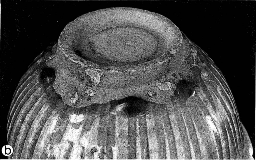
Pl. II. Glaze defects: a , crazing; b , pooling.
