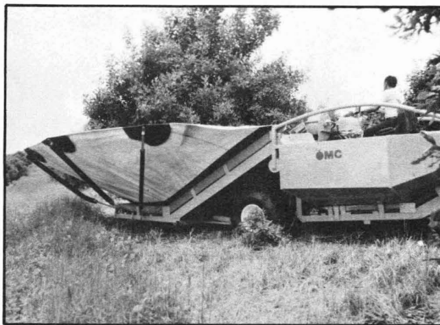
Fig. 20. Mechanical tree shaker in a macadamia field with a trunk grab and an apron catchment frame that possibly can be used for guava harvesting.
