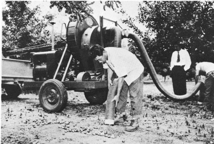
Figure 125. Experimental vacuum harvesting of macadamia nuts placed on ground at Keauu Orchard, 1953. Note quarry waste spread on ground to fill crevices. (Courtesy of Mauna Loa Macadamia Nut Corp.)
