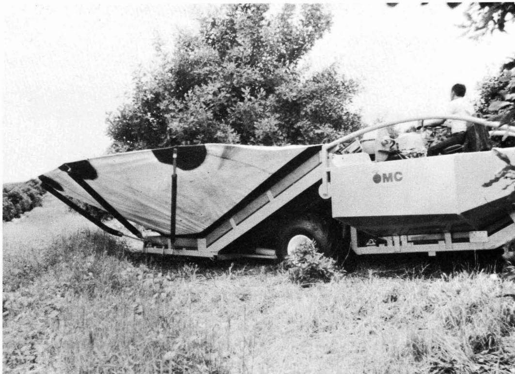
Figure 82. A shock wave harvester with its own catchment frame.
