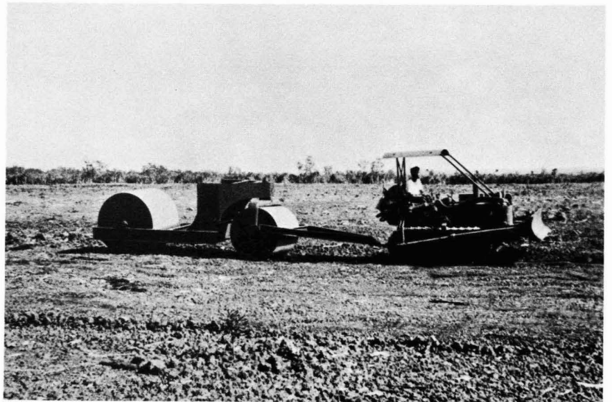
Figure 109. Land rolling at Keaau Orchard with a reclaimed steamroller, 1950. Note decided improvement in land surface. (Courtesy of Mauna Loa Macadamia Nut Corp.)
