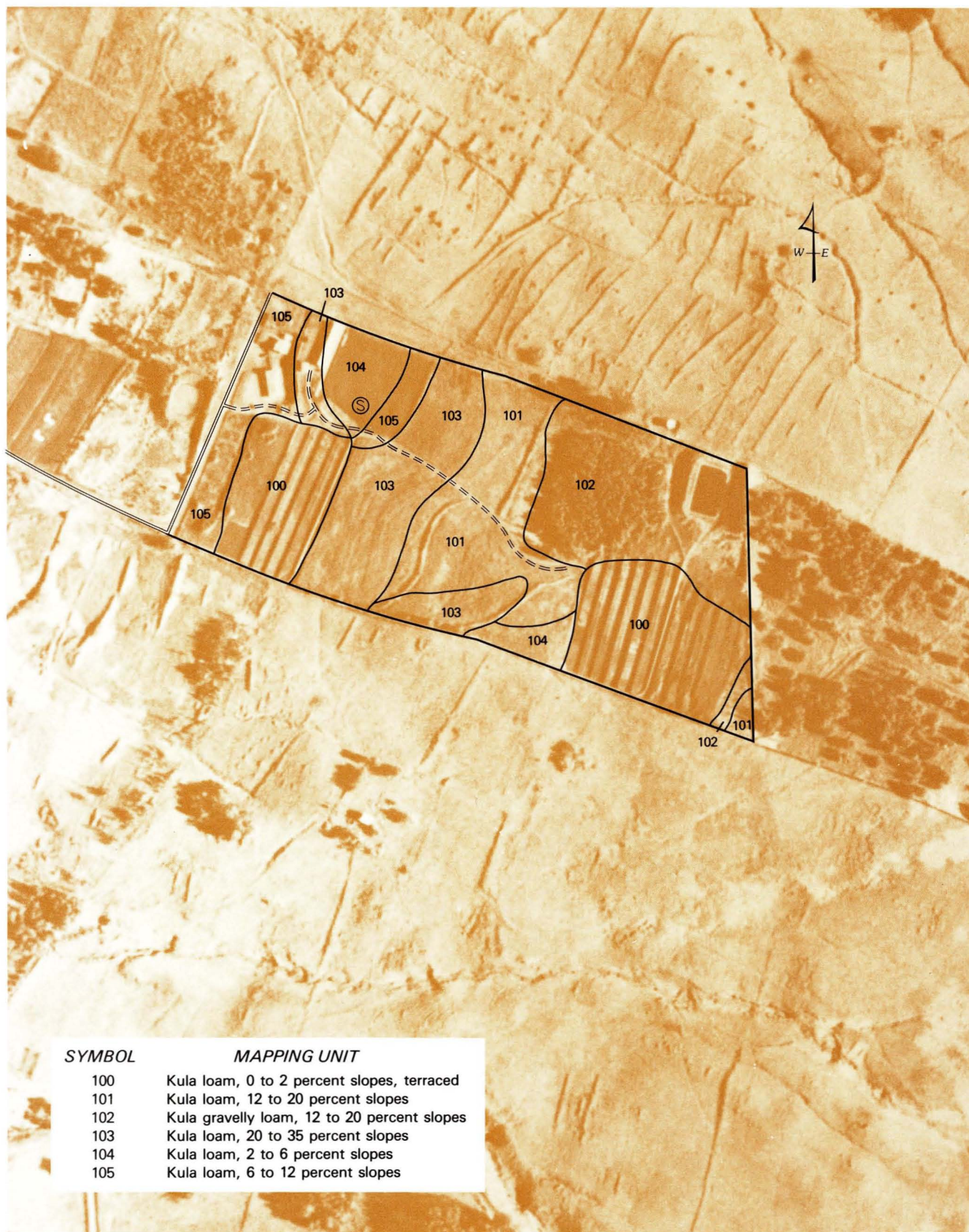
Fig. 6. Soil map of the Kula Experiment Station, Kula, Maui. Approximate scale: 1:4500. For general location, see Sheet 116, Soil Survey by Foote et al. (1972), lat. 20°45'45"N; long. 156°19'30"W.
