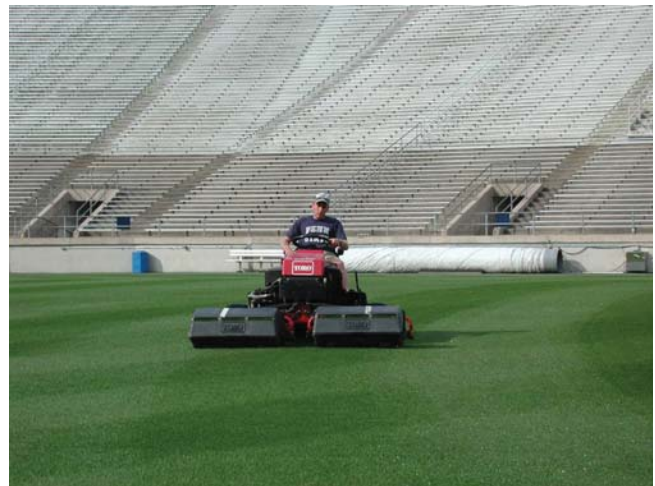
1. Reel-type mower (photo, P. Curtis)
