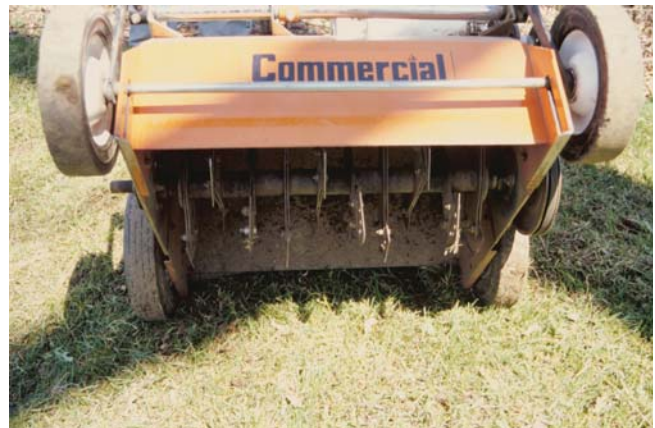
4. Vertical mower blades (photo, J.A. Borger)
