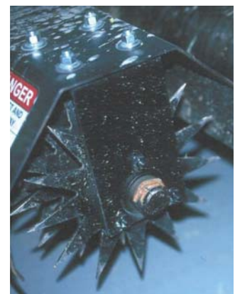
10. Spiking attachment for a power-driven reel mower (photo, A.S. McNitt)
