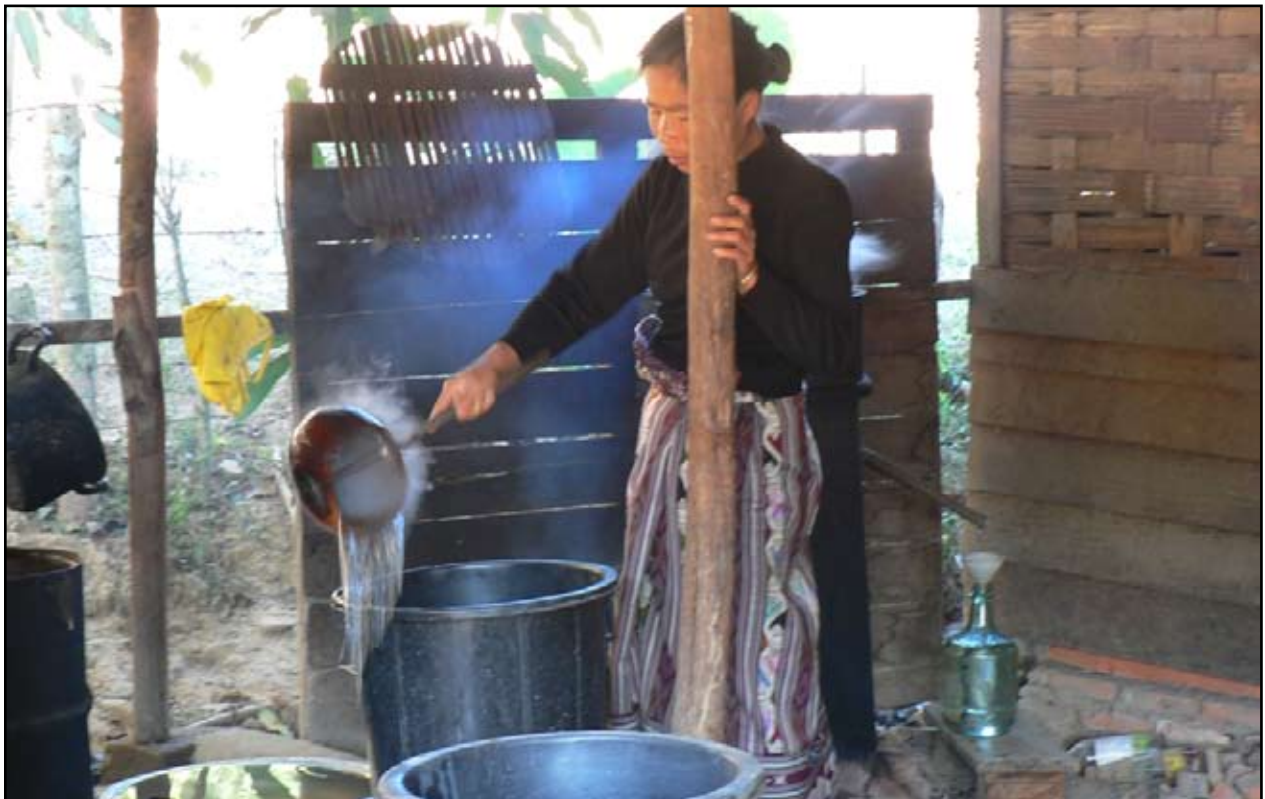
Figure 13. The hot water is regularly removed from the mo han...
